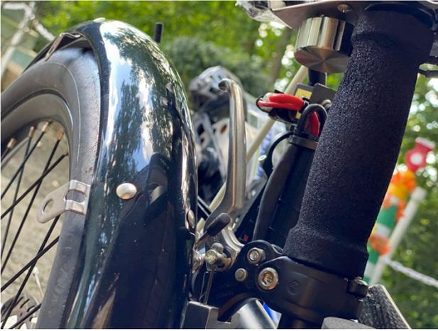
Regenerative braking volume ST is placed at the grip end.
