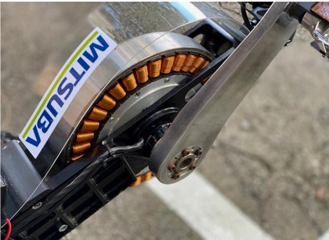
Pedal generator: MITSUBA prototype. Load adjustment is a digital dial type. Free choice according to the rider's leg strength.
