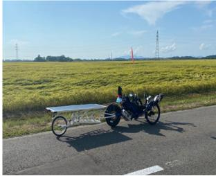
Maximum speed is  $50 \, \text{km} \, / \, \text{h}$ Optimal cruising speed is  $35 \text{-} 40 \, \text{km} \, / \, \text{h}$ In fine weather, 1 set of battery can run over  $100 \, \text{km}$
