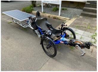
Seat is a racing kart type CFRP
