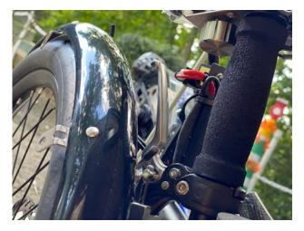
Regenerative braking volume ST is placed at the grip end.
